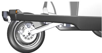
Now the swing arm will go further down and give access to the engine unit.
