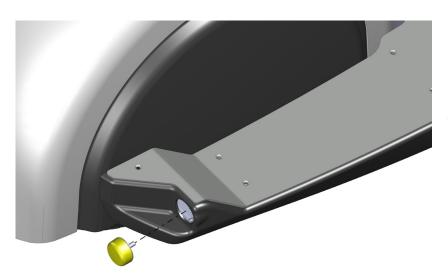
(3) Unplug the wires from the tail light. Unscrew it, pull it out and replace it. The indicator must be replaced as a unit.
