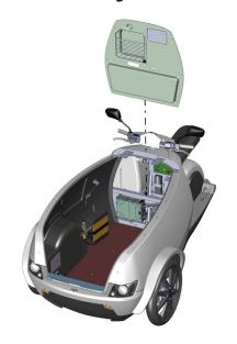
Remove the partition panel to gain access to the electronics.
