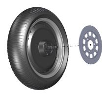
(7) Remove the braking disc and reuse it on the new engine. Use LockTite to secure the screws for the disc.
