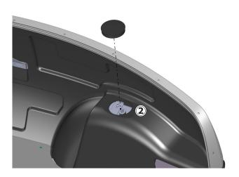
Remove the chock absorber cover in the boot and remove the upper chock absorber bolt ②.
