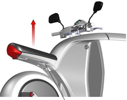
The seat height can be adjusted. Pull the seat adjustment handle and lift the seat to raise it. Push the seat to lower it. The handle will snap into place when released.
