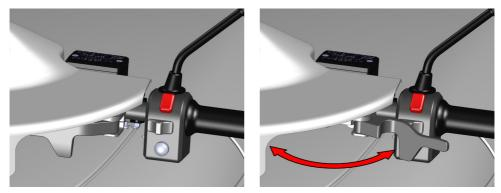
Pull out the handle to apply the parking brake.
