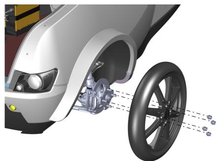
The front wheels can easily be removed and send to a workshop in case of a flat.
