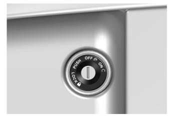
Switch off the vehicle by turning the key to OFF. Turn the key to PUSH and push it in. When the steering lock is engaged, turn the key to LOCK and remove it.
