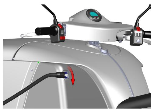
The charger connector must be turned 90° clockwise when inserted in the charger socket.
